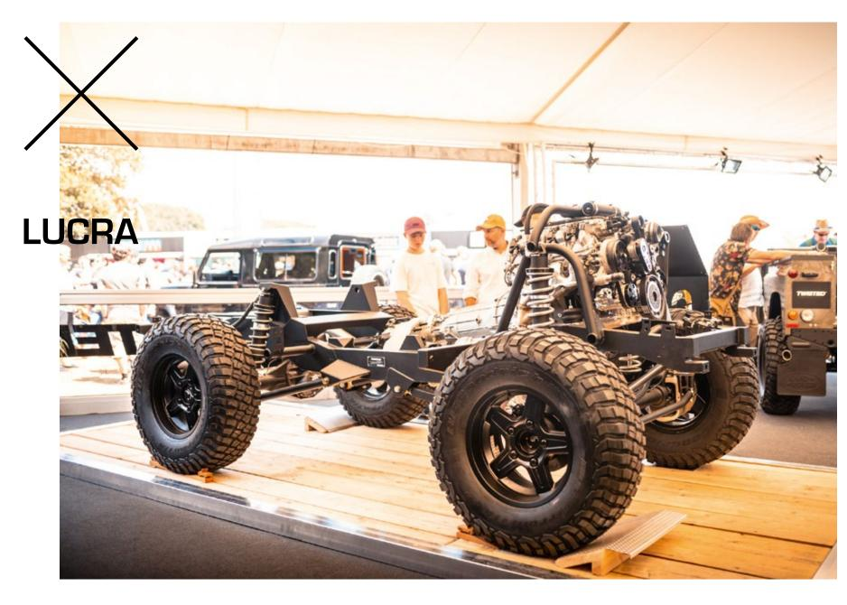
The driveline boasts a 6.2L GM Gen V LT4 supercharged, direct injection engine with 650bhp and 650 ft-lb of torque, Atlas 2 Speed transfer case and Wilwood six-piston front, four-piston rear vented disc brakes.
