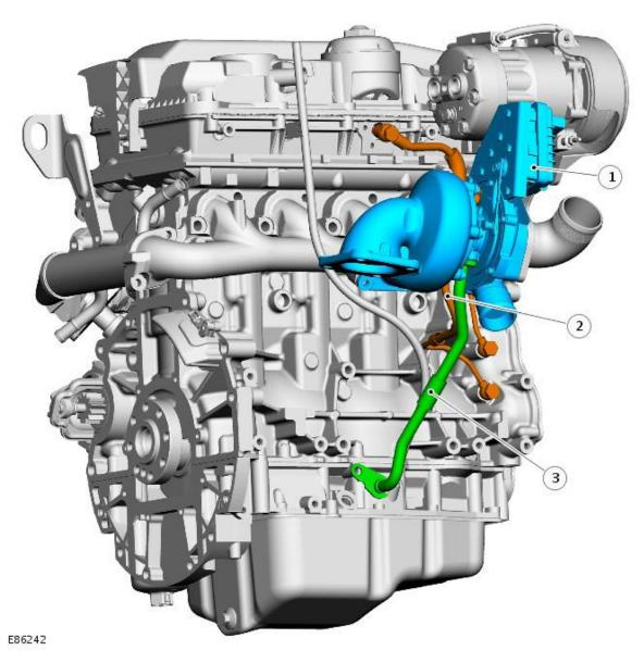
Turbocharger oil return tube bolts
