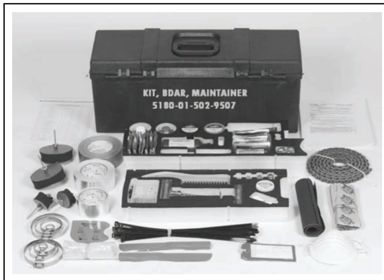
Figure A-2. Maintainer's BDAR kit
