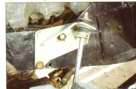
Rear shocks too are +5" Rough Country Units, again picking up on the chassis using Gwyn Lewis mounts
