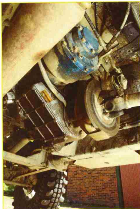
Original LT77 box and LT230 transfer case are from the same Discovery that donated its engine way back when. Bolted to the back of the latter are two things that make the vehicle a lot better off-road, in the shape of an Ashcroft underdrive and an X-Brake
