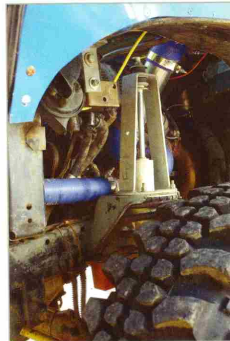
Rough Country +5" front shocks are mounted using towers from Gwyn Lewis
