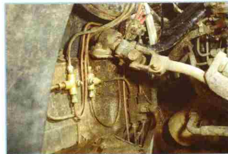
Brake servo from a 90 runs to dual inlet front calipers
