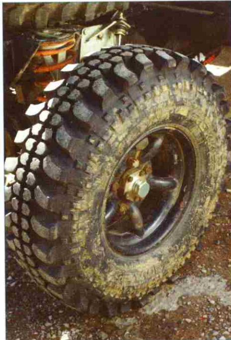
35x10.50R16 Simexes are mounted on max-offset Mach 5s, though the latter are slated for replacement with a set of beadlocks. Note also the Ashcroft drive members which turn the whole plot
